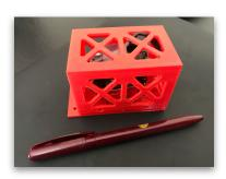
S4Arduino and S4Pi share the 1.5p PocketQube package. It is a 3D printed 5x5x7.5 cm plastic
